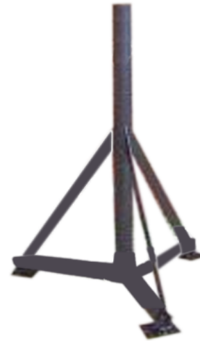
Ground Stand. Fully Welded 76mm dia pole. 1Mtr High. Including 3 adjustable feet
